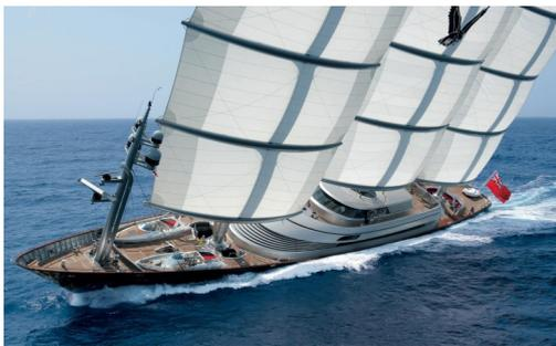
The Dyna-Rig is a balanced rotating modern rig specifically designed for large modern superyachts. Easy to use, and with no highly loaded lines on deck, it is one of the safest sailing systems available. Clean sail shapes and aerodynamic lines combine to create a highly efficient sailing rig on all points of sailing.
